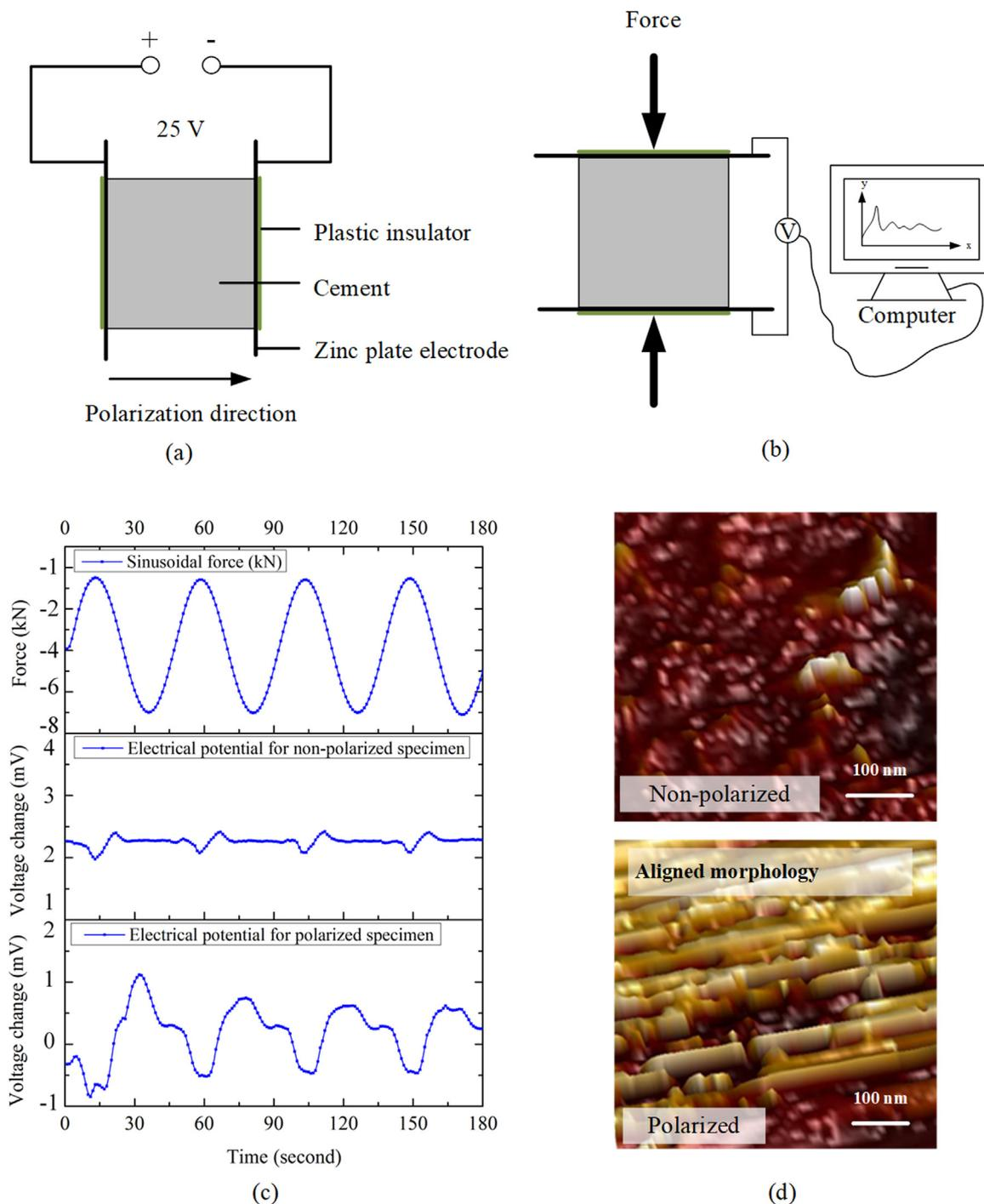
**Fig. 3.** Electrical treatment to improve cement piezoelectricity: (a) curing of cement paste under the electric field with the potential of 25 V, (b) polarized cement paste under compressive loading and measurement of the electrical signal, (c) the mechanical force and electrical signals between plain cement and polarized cement, and (d) the AFM result of plain cement and polarized cement.
