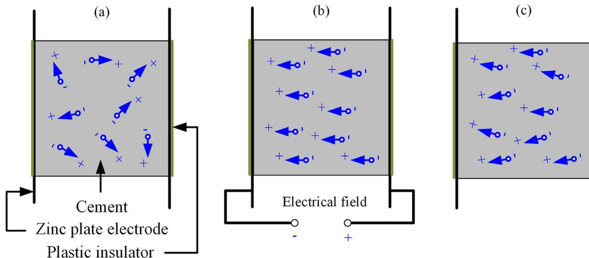
Fig. 2. Electrical treatment to improve cement piezoelectricity: (a) random orientation of electric dipoles prior to electric field exposure; (b) cement curing under the electric field treatment; (c) polarization in the cement paste remains after removing the electric field when the cement is hardened.
