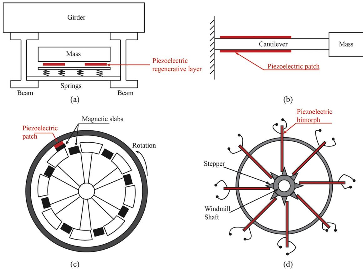
Fig. 5. Piezoelectric structural elements: (a) piezoelectric damper, (b) piezoelectric cantilever, (c) piezoelectric harvester, and (d) piezoelectric windmill.
