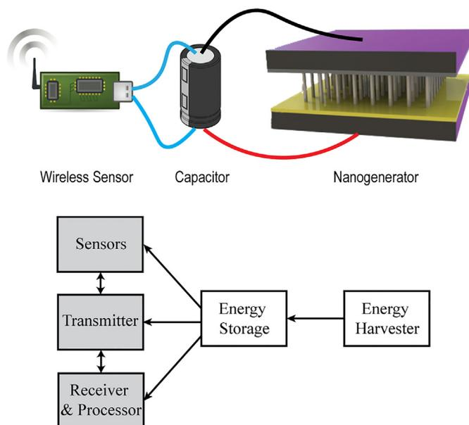
Fig. 4. Energy harvesting from piezoelectric generators and self-sustained sensors.
