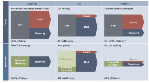
\* The efficiency of internal-combustion engines in other applications (e.g. maritime transport, engine-driven power plants) can exceed 50 %.
