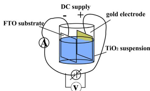
Fig. 9. Schematic of the electrophoretic deposition (EPD) setup [122].
