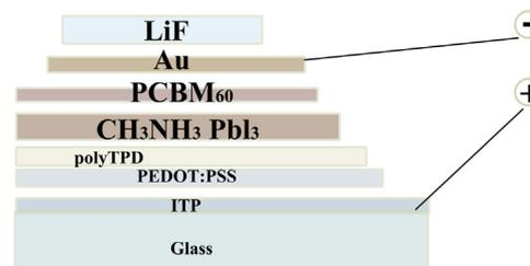
Fig. 7. Perovskite solar cell layers [112].
