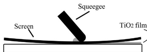
Fig. 3. Schematic diagrams of screen-printing polymer film [97].
