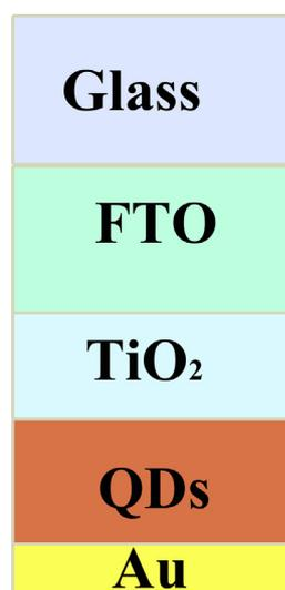
Fig. 10. Quantum dot (QD) solar cell [151].
