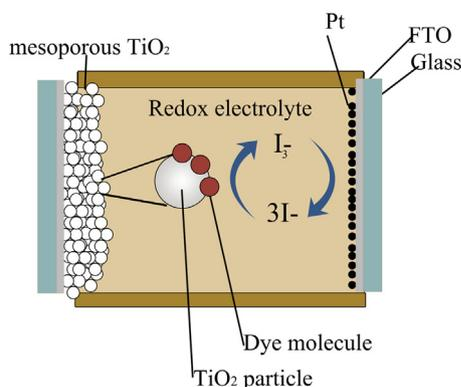
Fig. 2. Schematic overview of a dye-sensitized solar cell operational principle. [31].
