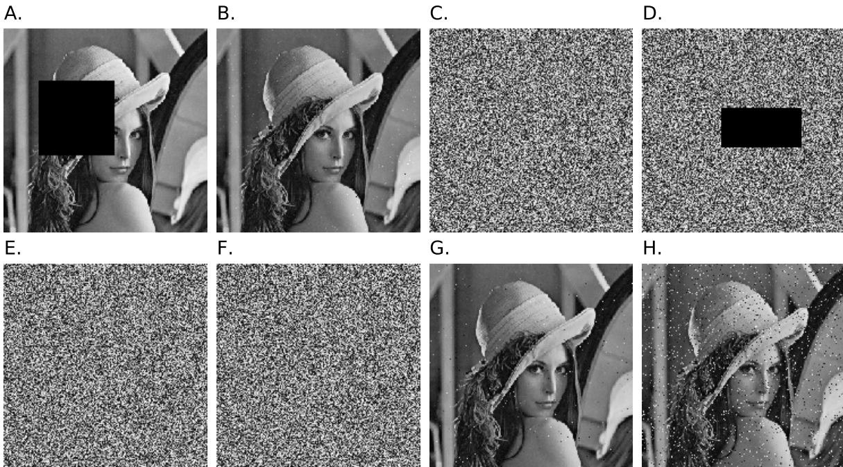
Figure 12: Manipulation Test: A) Some parts of source image is masked by zero values, B) White noise has been added to image, C) White noise has been added to Encrypted Image, D) Some parts of Encrypted image is masked by zero values, E,F) Encrypted images of A and B, G,H) Decrypted images of C and D
