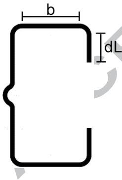
Figure B1: Flat widths of the flange ( $b$ ) and flange edge stiffener ( $dL$ ) of a channel with one intermediate web stiffener
