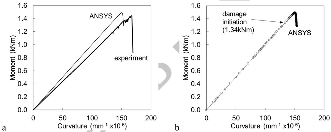
Figure 11: Finite element (ANSYS) solution for specimen flax 4 layers 2WS LL; a) comparison with experimental moment-curvature response, b) ANSYS solution points and damage initiation
