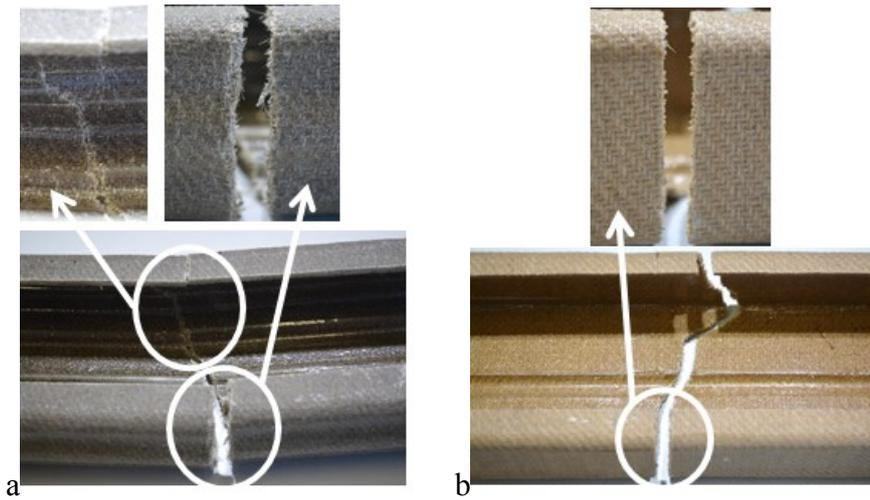
Figure 8: Exemplar failure modes (tension flange is the lower flange); a) 6 layered flax, b) 4 layered jute
