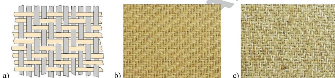
Figure A1: 2x2 Twill weave fabric: a) generic pattern, b) Biotex Jute 400g/m<sup>2</sup> c) Biotex Flax 400g/m<sup>2</sup>
