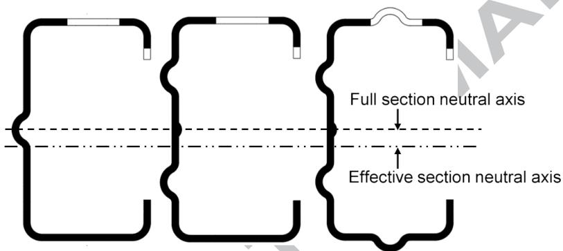
Figure 9: Exemplar effective widths (black areas) at the limit state, and the shift of the major axis bending neutral axis (towards the tension side) between the full section and the effective section
