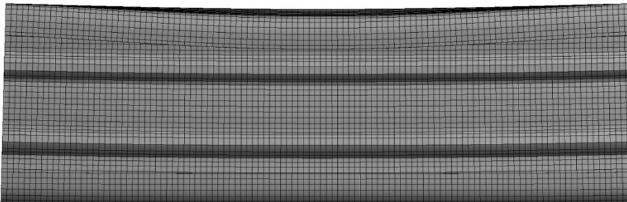
Figure 12: Exemplar deformation at the ultimate state (true scale); flax 4 layers 2WS SL
