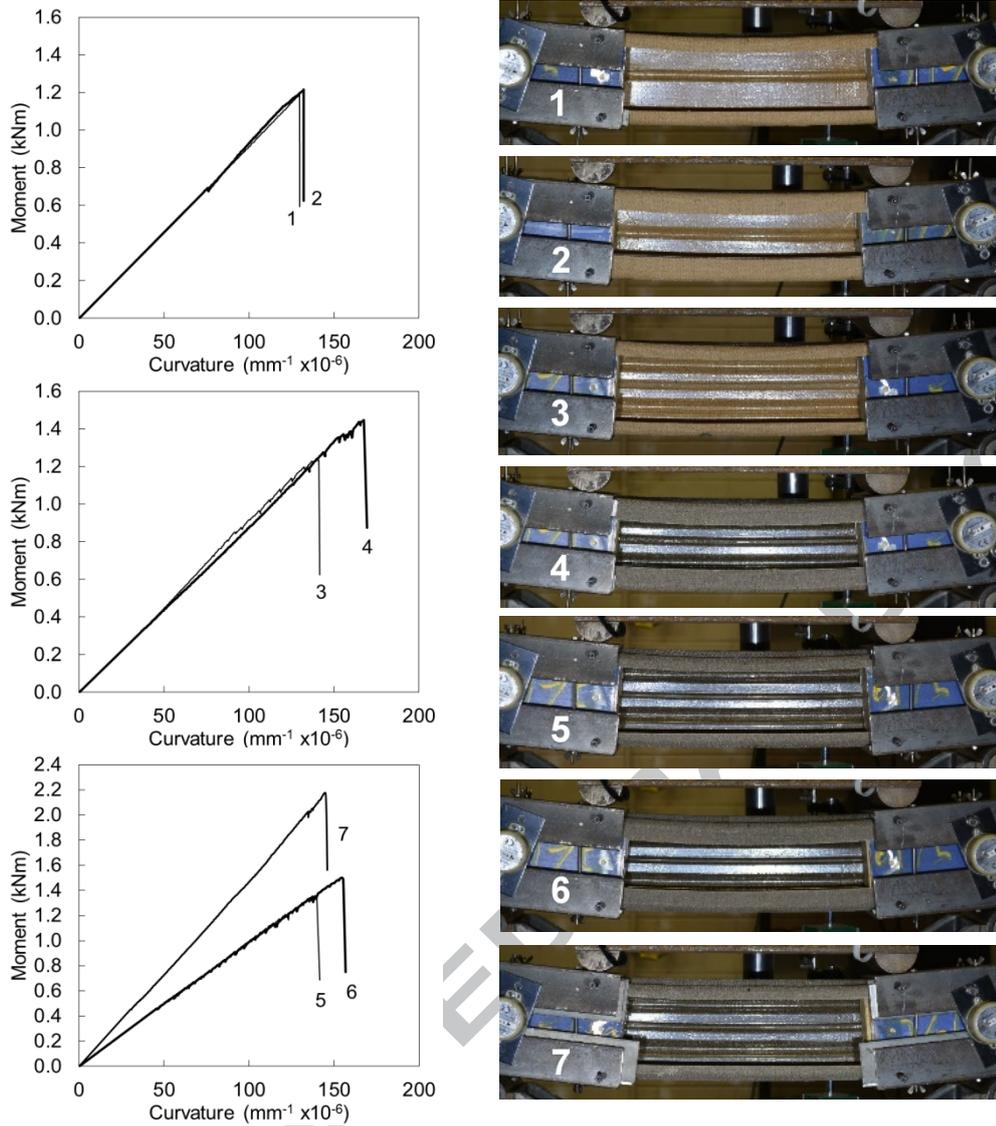
Figure 7: Moment-curvature responses of exemplar channels with photographs approaching the ultimate state; 1) jute 4 layers 1WS SL, 2) jute 4 layers 1WS LL, 3) jute 4 layers 2WS SL, 4) flax 4 layers 2WS LL, 5) flax 4 layers 2WS 1FS SL, 6) flax 4 layers 2WS 1FS LL, 7) flax 6 layers 2WS 1FS SL
