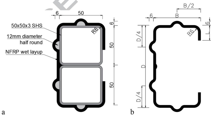
Figure 3: Channel fabrication; a) exemplar fabrication mandrel, b) resulting channel section ( $B$ ,  $D$ ,  $L$  are outside dimensions)
