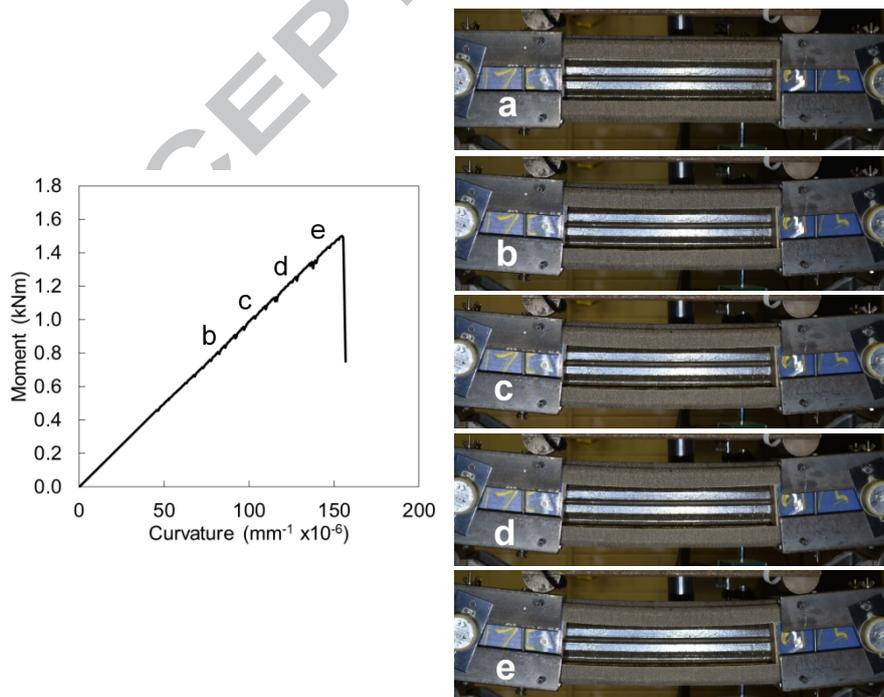
Figure 6: Exemplar moment-curvature response (flax 4 layers 2WS 1FS LL) with photographs at periodic intervals; a) 0kNm, b) 0.88kNm, c) 1.13kNm, d) 1.25kNm, e) 1.44kNm
