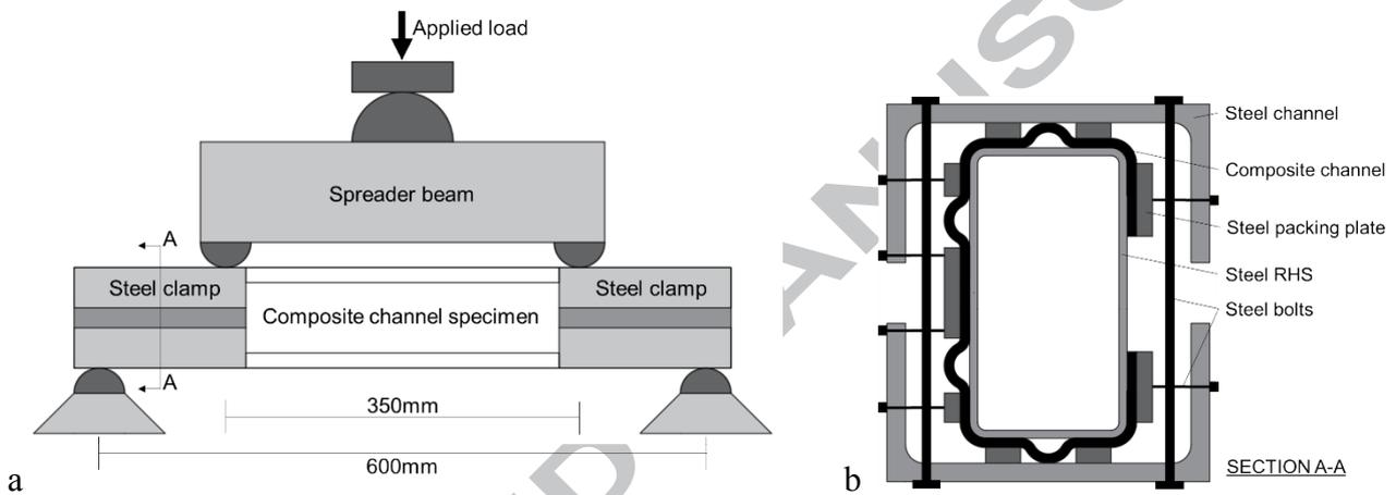
Figure 5: Experimental four-point bending setup; a) elevation, b) section
