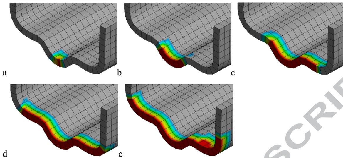
Figure 13: Exemplar progression of damage (jute 4 layers 2WS 1FS LL); a) 1.385kNm, b) 1.399kNm, c) 1.401kNm, d) 1.380kNm, e) 1.349kNm (red is fully damaged, grey is no damage)
