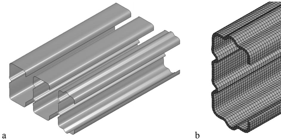
Figure 10: ANSYS modelling; a) exemplar finite element model geometries, b) exemplar 3mm shell mesh used in all models
