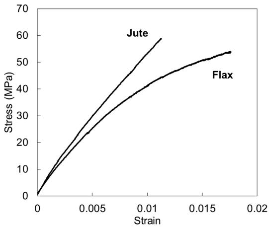
Figure 1: Measured uni-axial tension stress-strain curves (fibre volume fractions of 39% for jute, and 40% for flax)
