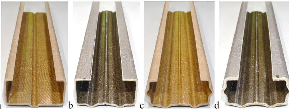
Figure 4: Exemplar composite channel specimens: a) 4 layered jute (type Figure 2a); b) 4 layered flax (type Figure 2d); c) 4 layered jute (type Figure 2e); d) 6 layered flax (type Figure 2f)
