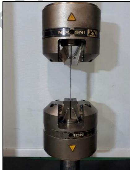
Fig. 9 Tensile test of a single-lap joint specimen.
