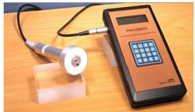
**Fig. 2.** The Adek™ Percometer and the probe.
