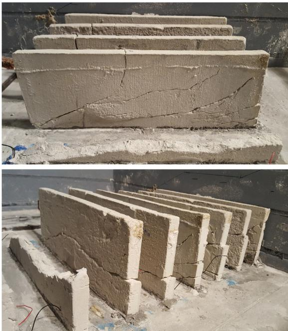
Fig. 4. Post-test excavation photos of the soil-cement panels (toe of berm is to left side of photos).
