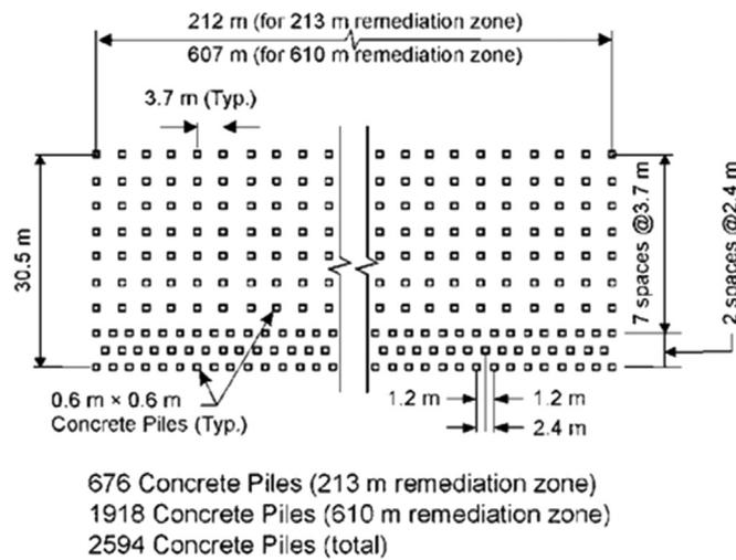
Fig. 6. Plan view of pile remediation of Sardis dam [1].
