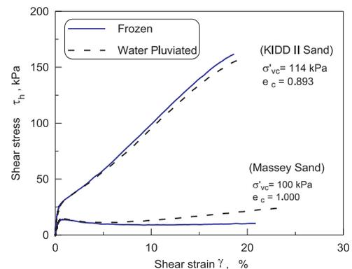
Fig. 17. Comparison of stress-strain curves from frozen specimens and from water pluviated specimens [16].
