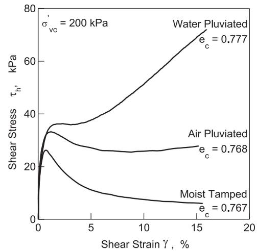
Fig. 16. Effect of stress path on stress-strain response [16].
