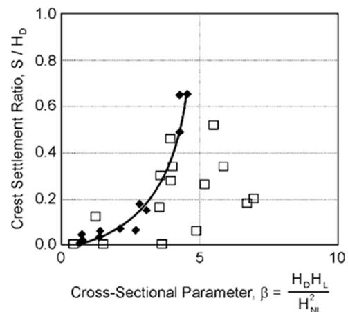
Fig. 12. Comparison of post-earthquake observed settlements for all slopes with predicted settlements.
