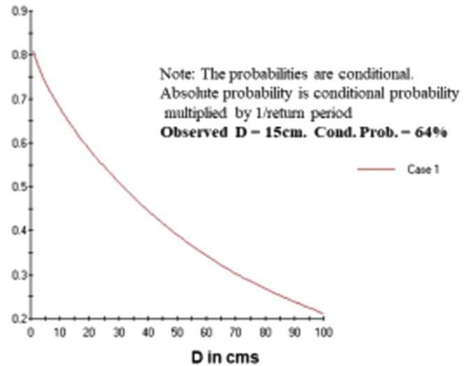
Fig. 9. Conditional probabilities of displacements in Lexington Dam slopes during Loma Prieta Earthquake.
