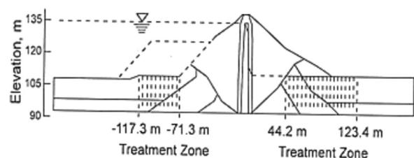
Fig. 13. Cross-section of MIAD showing treatment zones.
