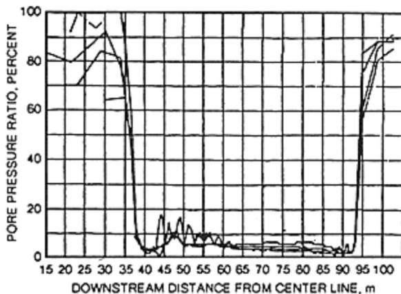
Fig. 15. Pore water pressures around the treatment zone.
