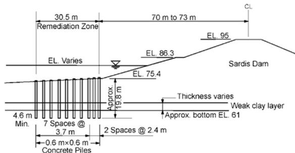
Fig. 5. Elevation of pile remediation of Sardis dam [1].
