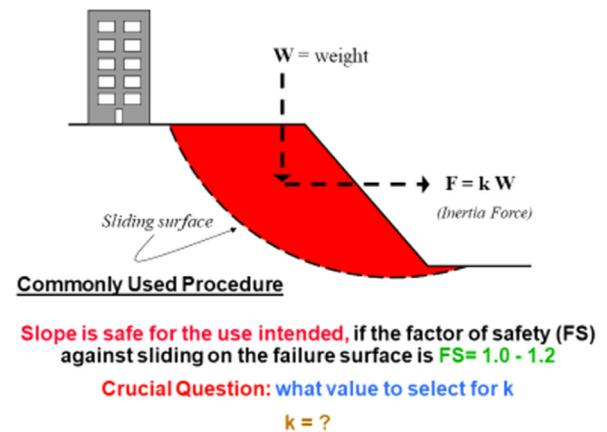
Fig. 7. Mechanism for pseudo-static slope analysis.
