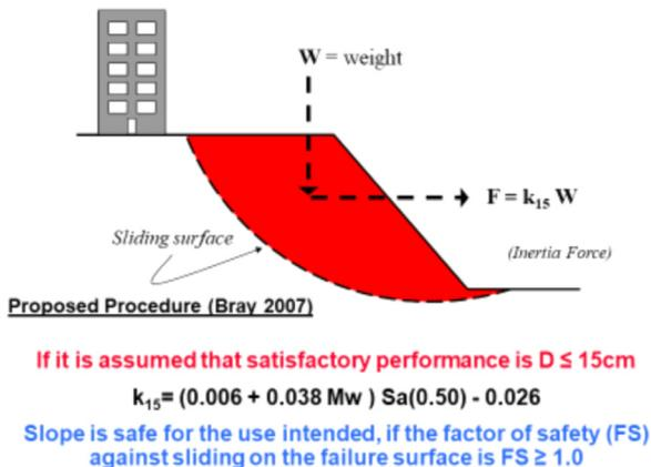
Fig. 8. Mechanism for pseudo-static analysis using  $k_{15}$ .
