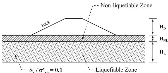
Fig. 10. Typical cross-section of dike used in parametric studies.
