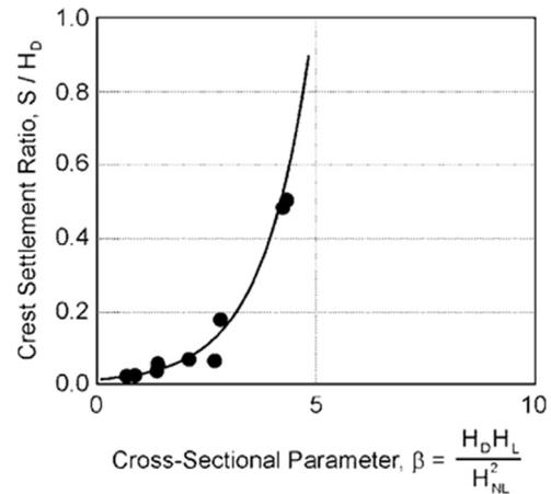
Fig. 11. Comparison of computed settlements with the black prediction curve.
