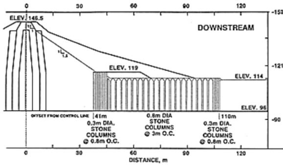
Fig. 14. Details of the downstream remediation plug.
