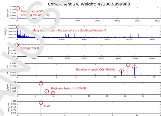
Figure 6: A component from the decomposition of an “extended time independent connections” tensor, clearly identifying suspicious ICMP traffic.
