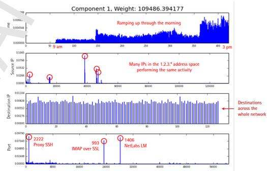
Figure 3: A component from the decomposition of an “incoming traffic” tensor. The component represents distributed network mapping and port scanning with strong likelihood of hostile intent.
