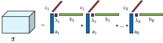
Figure 1: A CP Decomposition of a 3-dimensional tensor into  $R$  components.
