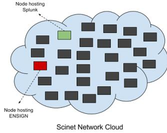
Figure 8: Pictorial representation of SCinet cloud infrastructure and deployment of CANDID/ENSIGN in the cloud.
