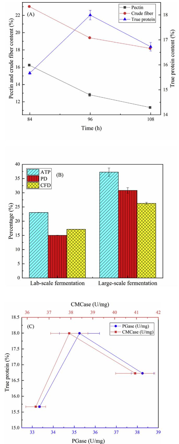
**Fig. 6.** The SCP feed quality of large-scale fermentation on orange waste. (A) The change of true protein, pectin and crude fiber content over time. (B) The comparison of ATP, PD, CFD by large-scale fermentation and lab-scale fermentation. (C) The relationship between PGase, CMCase and true protein. (For interpretation of the references to color in this figure legend, the reader is referred to the Web version of this article.)
