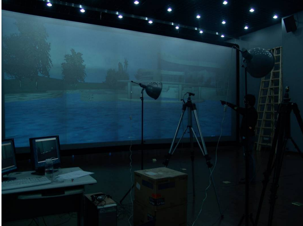
Fig.1: A large screen presenting the virtual environment which is produced by a multi-projector system.
