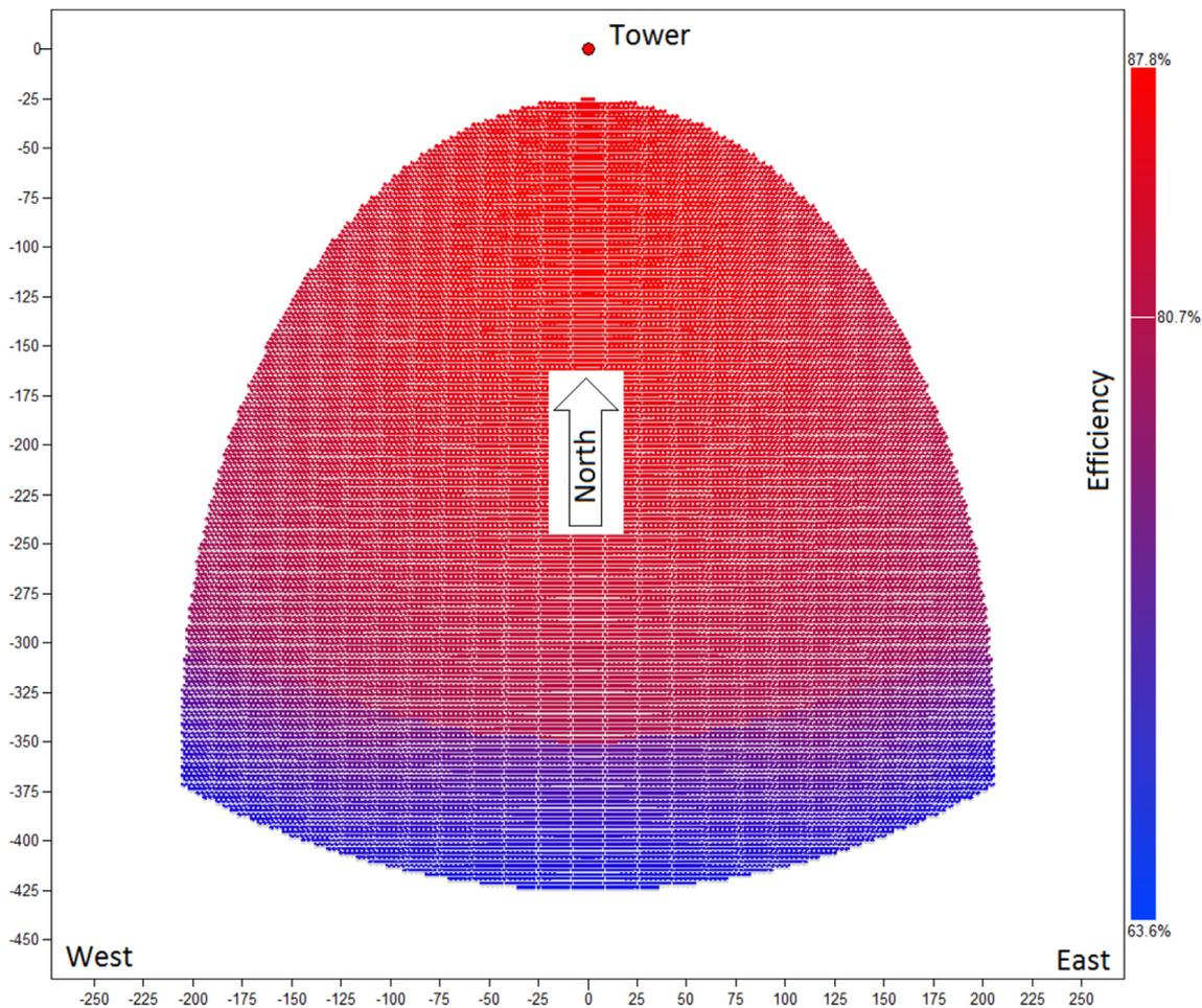
Fig. 5 – Heliostat field lay-out for downward inclined cavity receiver.
