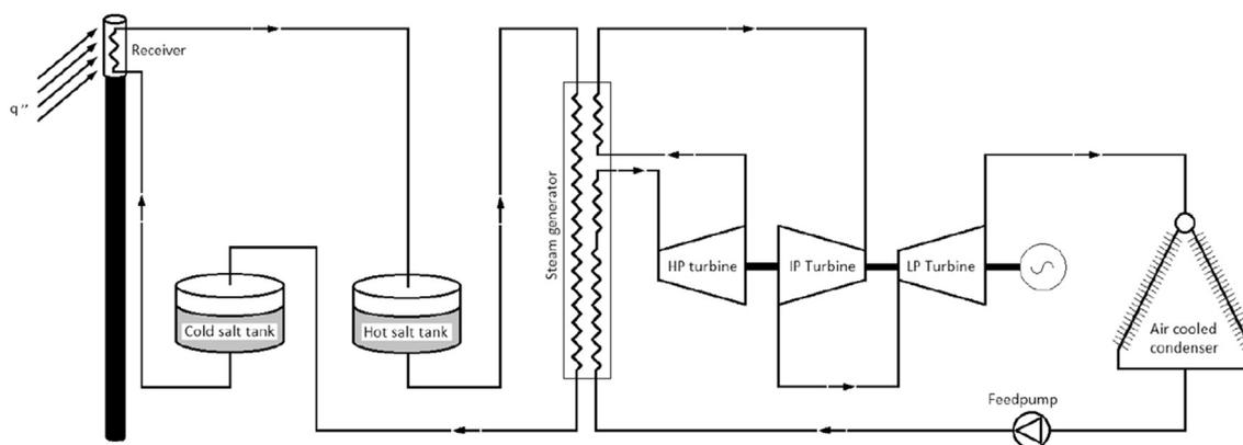
**Fig. 3 – Conventional molten salt central receiver plant.**
