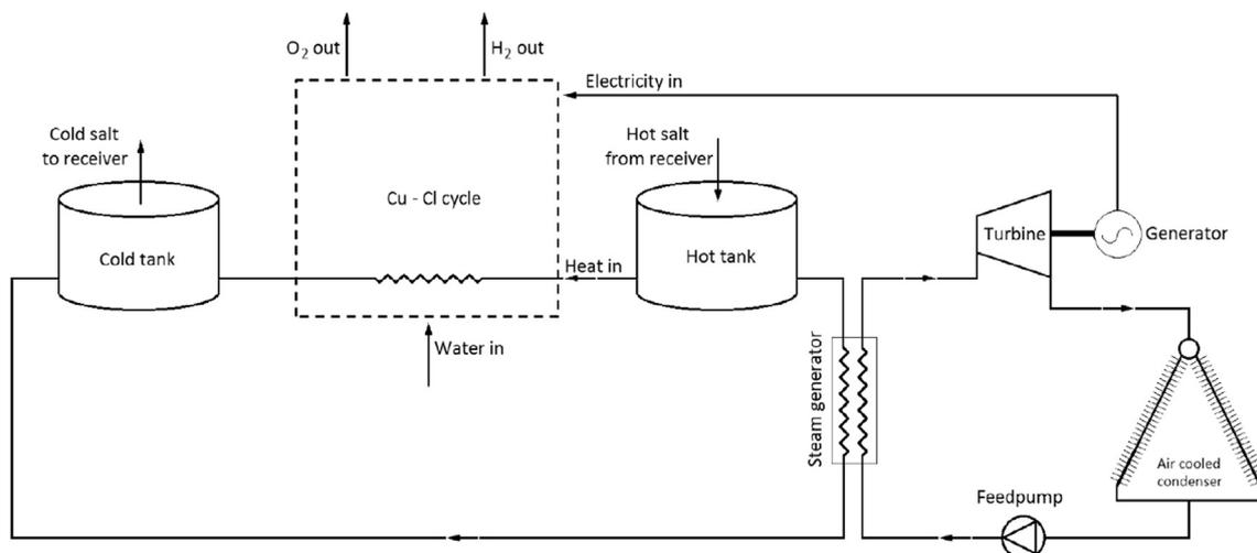
Fig. 7 – Process flow diagram for integration combined cycle solar thermal power and process heat plant with Cu–Cl thermochemical water splitting cycle.
