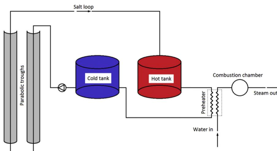
Fig. 1 – Parabolic trough plant supplying solar preheating to methane/steam reforming plant.
