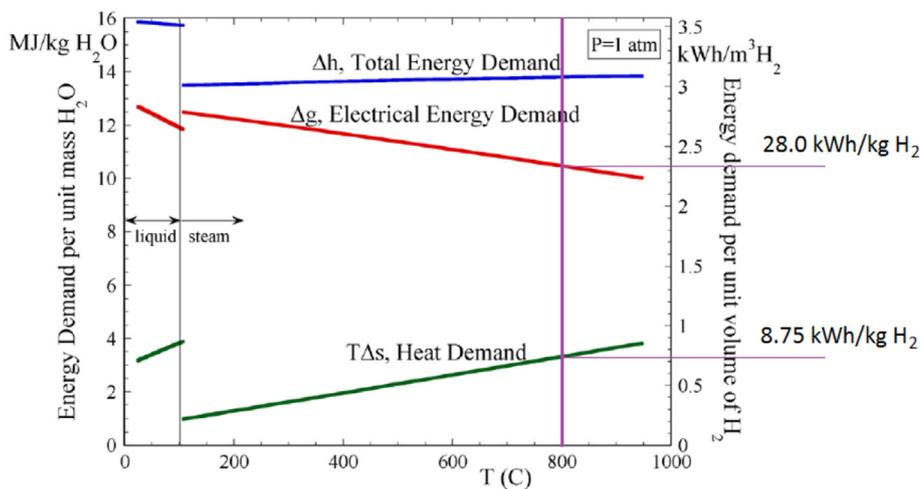
Fig. 6 – Energy requirement of high temperature electrolysis as a function of temperature [13].
