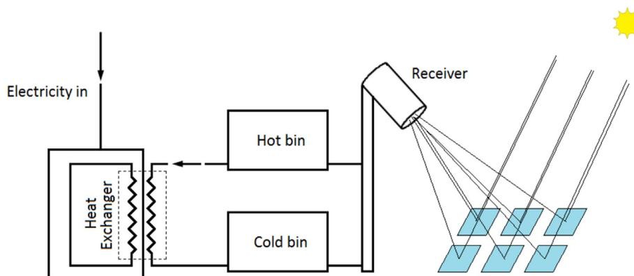
**Fig. 4 – Proposed solar energy supply electrolysis plant for temperatures over 800 °C.**
