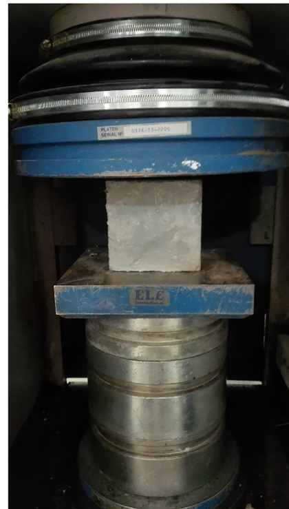
Fig. 14. Compression test setup.
