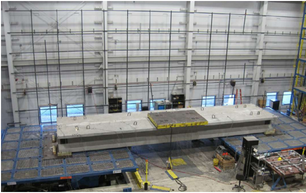
Fig.13. Set-up of Shake Table Test.
