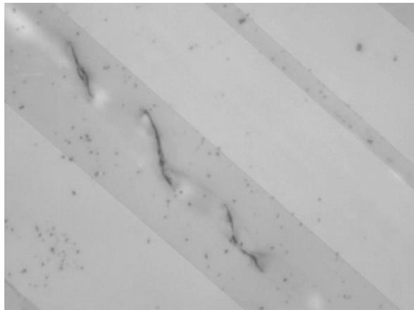
Fig. 2. Example of inclined inter-fiber micro-cracks in the matrix of a  $45^\circ$  ply [3]
