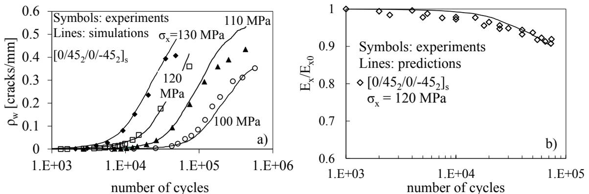
Fig. 4. Predicted and experimental trends of a) the crack density evolution and b) the stiffness degradation
