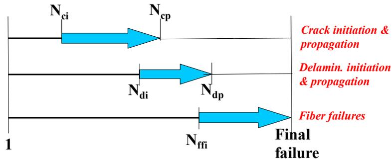
Fig. 1. Schematic of the damage evolution e modelling strategy for the life assessment of composite laminates
