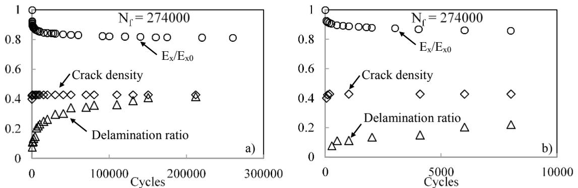
Fig. 5. a) Normalized Young modulus, crack density and delamination ratio for a glass/epoxy [0/90<sub>2</sub>], laminate tested with a global laminate stress of 120 MPa; b) zoom of the first 10000 cycles
