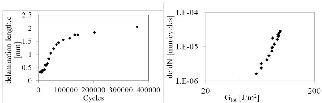
eventually related to the delamination growth rate. It was thus possible to define a Paris-like curve (Figure 6b) relating the growth rate to the mode II energy release rate (the mode I contribution is very limited or absent, at least under tensile loadings). This approach allows the delamination length to be predicted as a function of the number of cycles.
