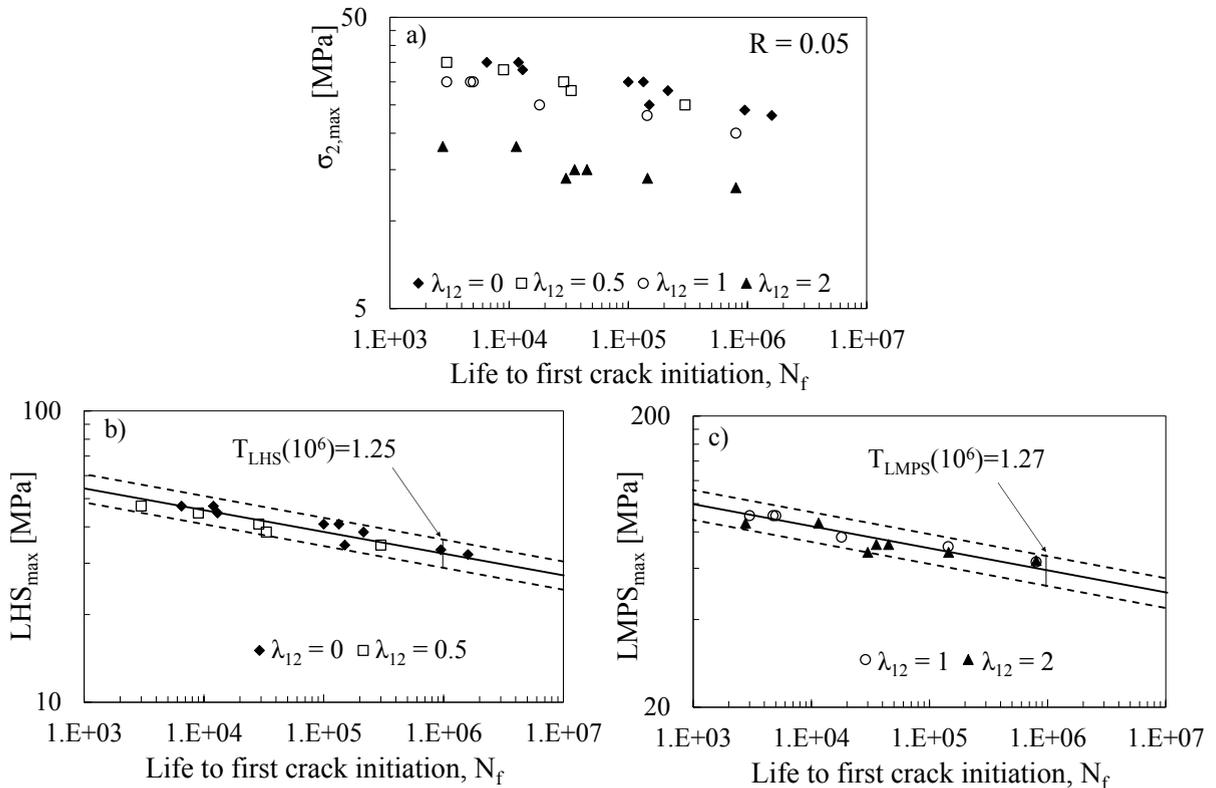
Fig. 3. First crack initiation results for glass/epoxy tubes [2]: maximum a) cyclic transverse stress, b) LHS and c) LMPS against the number of cycles for first crack
