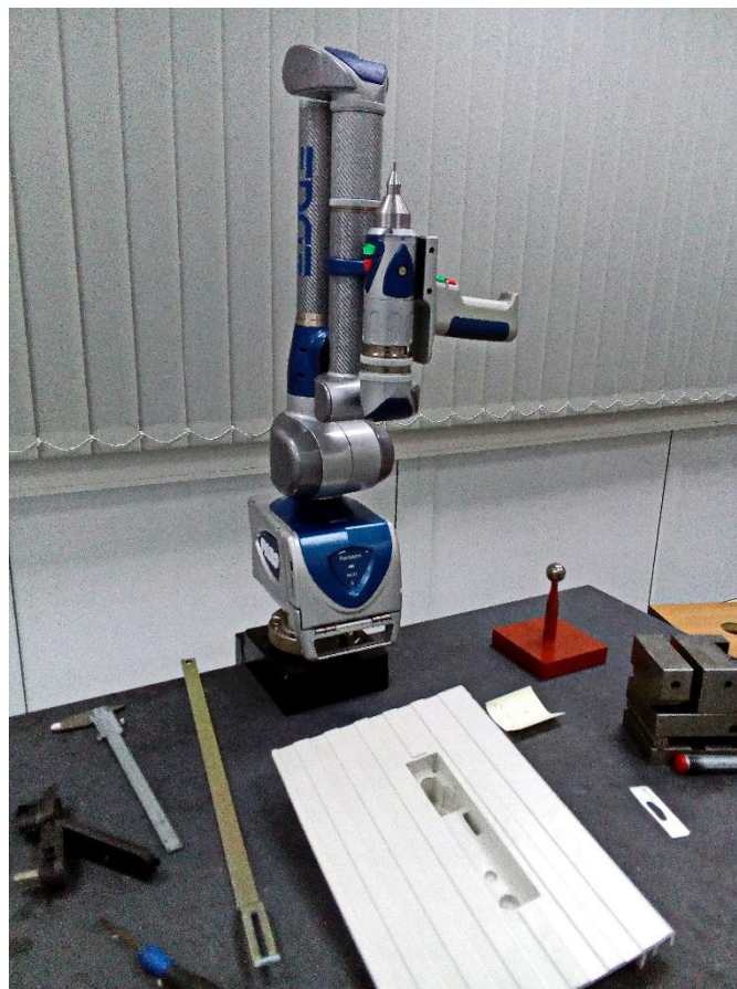
Fig. 5. The FaroArm Edge® polyarticulate arm, along with the laboratory stand.
