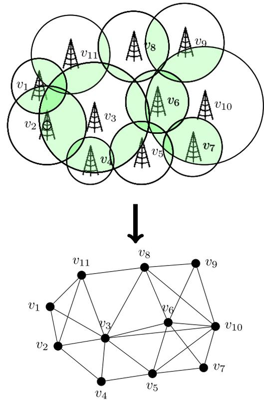
**Fig. 3.** System Model: Graph construction based on antennas positions and interferences.
