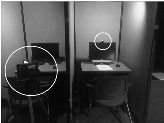
Fig. 1. Pictorial representation of the experimental set-up. Note the illumination on both the webcam (right) and the video recorder (left), outlined in white.
