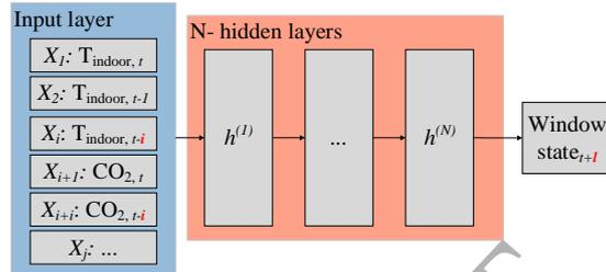
Figure 1: Learning procedure overview. The sequences of measured indoor climate and the data from the last time-step  $t$  are defined as the model inputs. The duration of the input sequences  $i$  (red color symbol) is defined as additional hyperparameter. Eventually, the relationship between the predictive performance and the time lag of prediction  $l$  (red color symbol) is analyzed.
