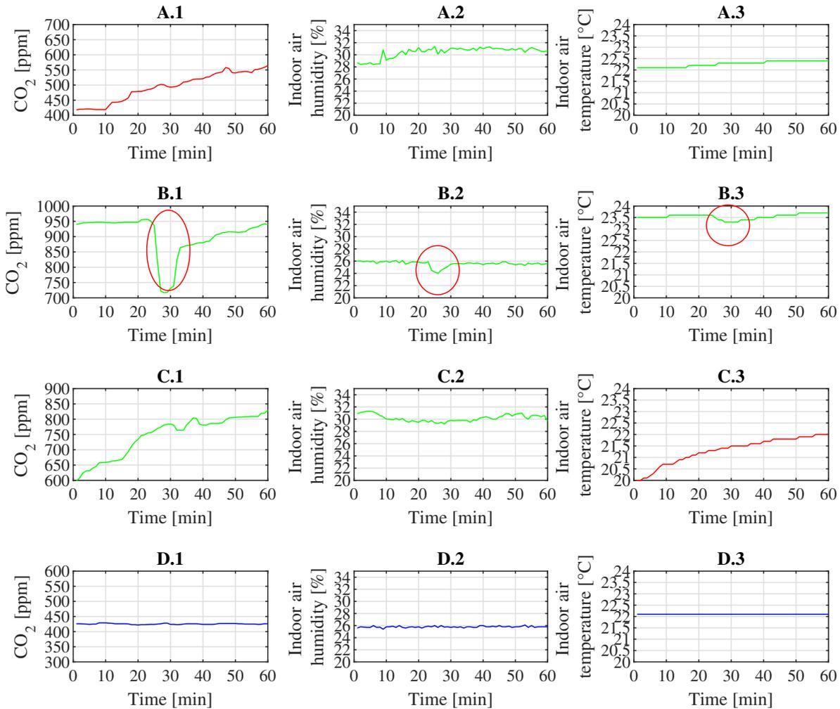
Figure 9: Changes in the indoor climate prior over one hour, where the window states were correctly predicted to be opened.
