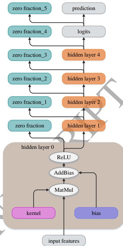
Figure 4: Visualization of the developed neural network. The graph notation corresponds to notation as used in Tensorboard [45].
