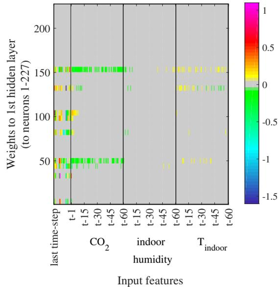
Figure 7: Magnitude of the weights from the input layer (x-axis) to the neurons first hidden layer (y-axis). For the visualization purpose, the bars representing the weights of higher absolute magnitude (colored fields) are enlarged vertically by the factor 6.
