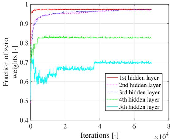
Figure 6: Fraction of the weights set to zero during model training.
