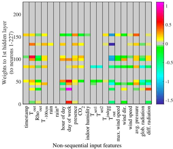
Figure 8: Magnitude of the weights from the input features that refer to non-sequential data, to the neurons in the first hidden layer. For more detailed description of the input features, the reader is referred to [33].
