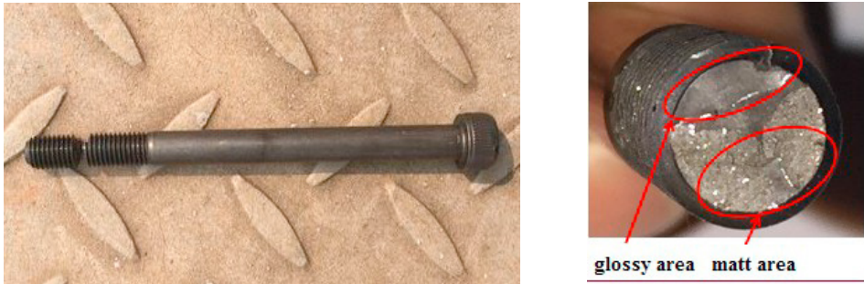
Fig. 2. (a) Macro morphology of motor energy storage bolt; (b) Macro morphology of section.
