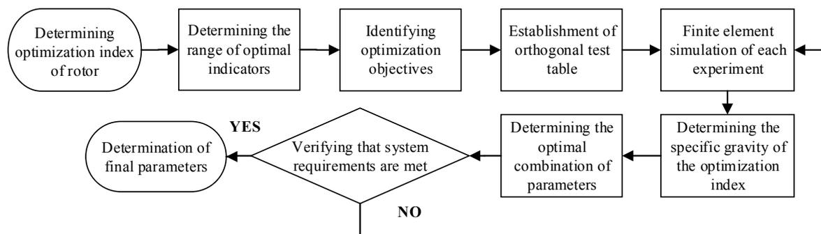
Fig. 2. Technical route diagram for optimization of Taguchi algorithm.
