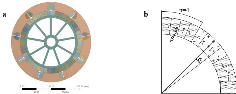
Fig. 1. (a) Cross section structure of motor; (b) Parameter diagram of Halbach array rotor.
