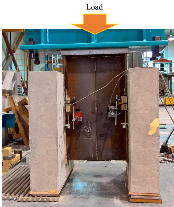
Fig. 6. Push test setup.
