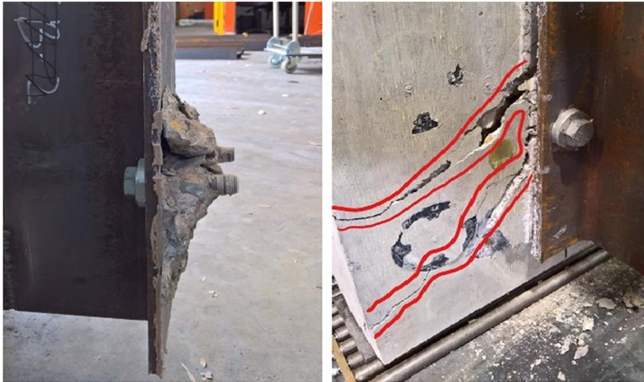
Fig. 16. Concrete break-out for specimen H2.
