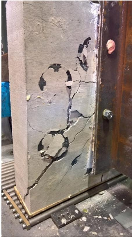
Fig. 19. Significant cracking in specimen S5.
