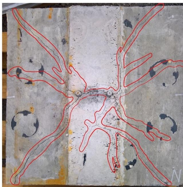
Fig. 15. Concrete splitting failure for specimen S1 (After demounting).
