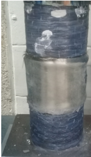
Fig. 11. Failure mode of the partially wrapped specimen.
