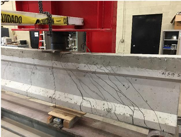
Fig. 16. Final cracking for individual scale girder test.
