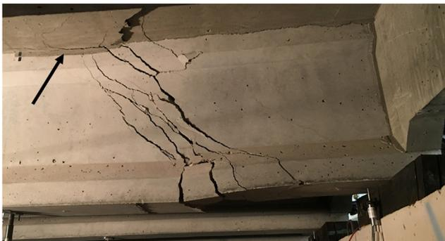
Fig. 14. Cracking in girder B at failure. Arrow indicates load location and punching shear.
