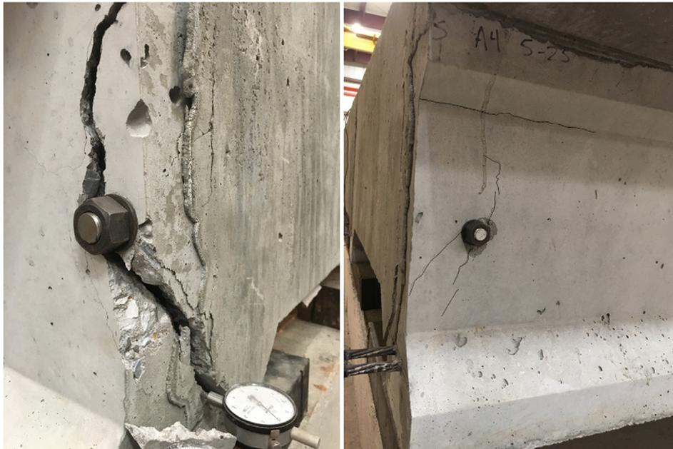
Fig. 13. Cracking at diaphragm to girder connections on girder A. Left image shows end closest to load, right image shows end farther from load.
