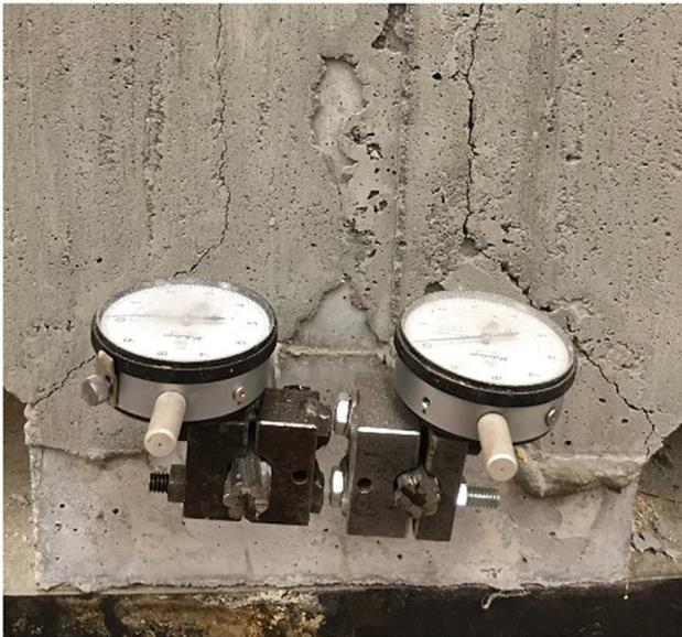
Fig. 10. Diaphragm-girder interface cracking prior to bridge test.
