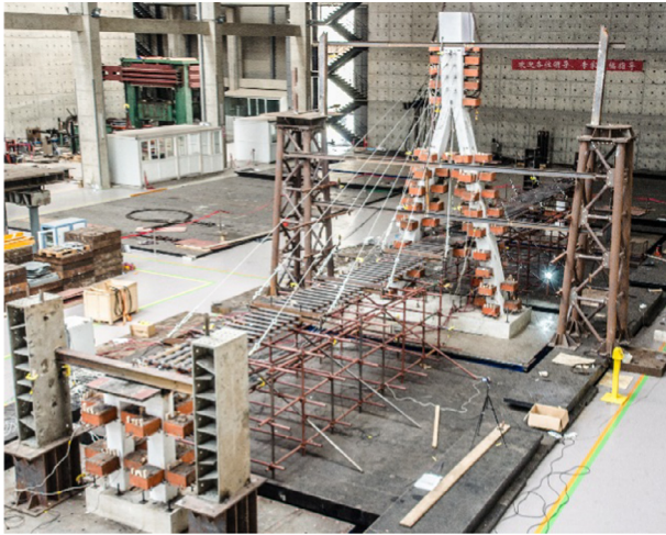
Fig. 5. Photo for full-bridge of the test model.
