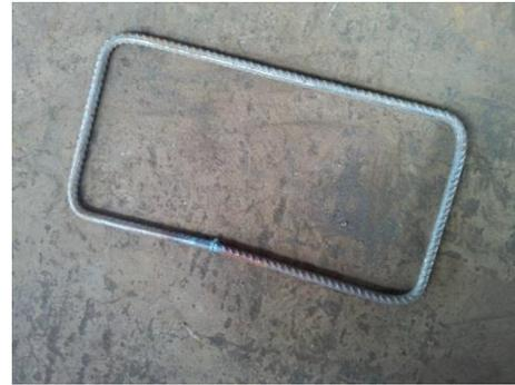
Fig. 3. Welded confinement steel hoop.
