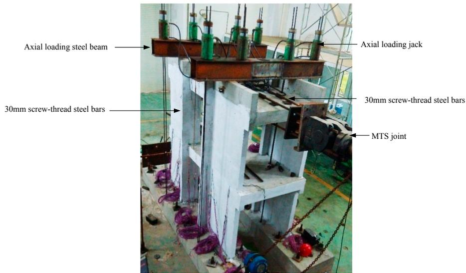
Fig. 18. Test setup and specimen in reality.
