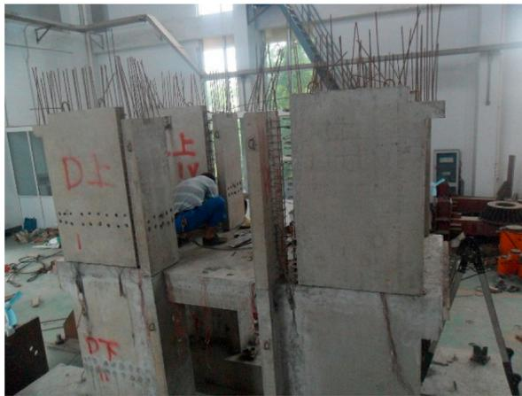
c. Component assembly of second floor
