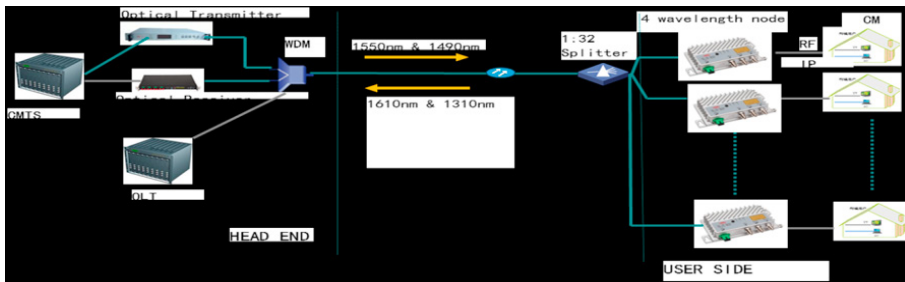
Fig2.a single-fiber four-wave FTTH fusion network topology
