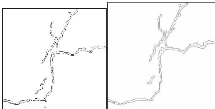
(a) Contour extraction of the canny algorithm (b) Contour extraction of the improved algorithm
