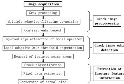
Fig. 1. The detection process of image cracks on concrete Bridges
