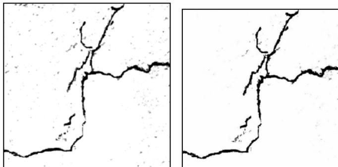
(a) primary filtering and enhancement (b) three groups of multi-window filtering and enhancement
