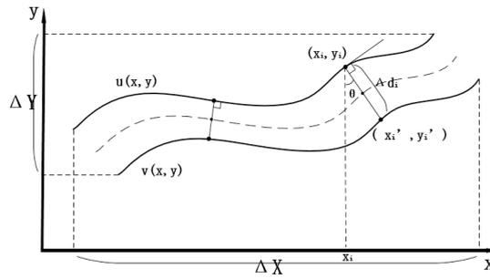
Fig. 5. The data detection of crack edge
