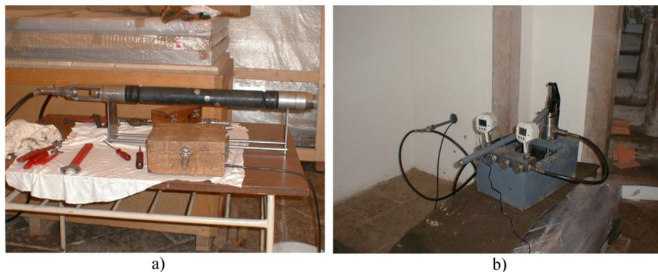
Fig. 15. BHD tests: a) dilatometer probe; b) hydraulic pressure pump and control unit.
