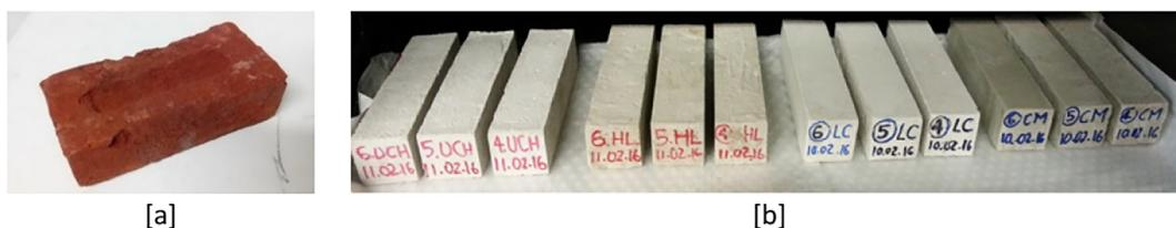
**Fig. 1.** Visual aspect of [a] Red Clay Brick (RCB) and [b] Mortar specimens (CM – LC – LH – HL). (For interpretation of the references to colour in this figure legend, the reader is referred to the web version of this article.)
