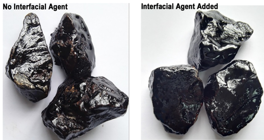
Fig. 15. Effect diagram before and after the improvement of adhesion between emulsified asphalt and granite.
