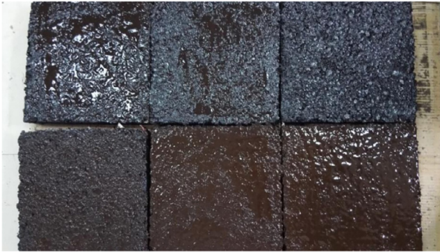
Fig. 8. Specimens Sprayed with Different Quantities of Hydrophobic Emulsified Asphalt.
