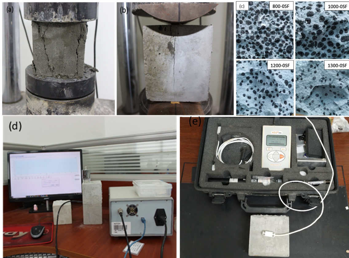
Fig. 3. Testing setup for (a) compressive strength (b) splitting tensile strength (c) Distribution of ECA in LAFC sample (d & e) thermal properties measurements with TC300E and Decagon KD2 Pro.
