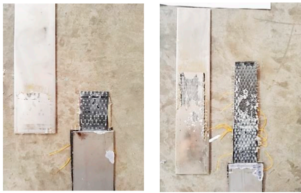
(a) Interface damage of completely debonding (b) Interface damage of mixed damage
