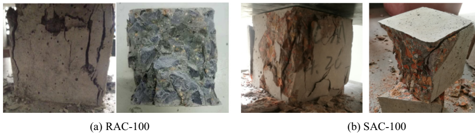
Fig. 7. Compressive failure modes of different varieties of coal gangue coarse aggregate concrete.
