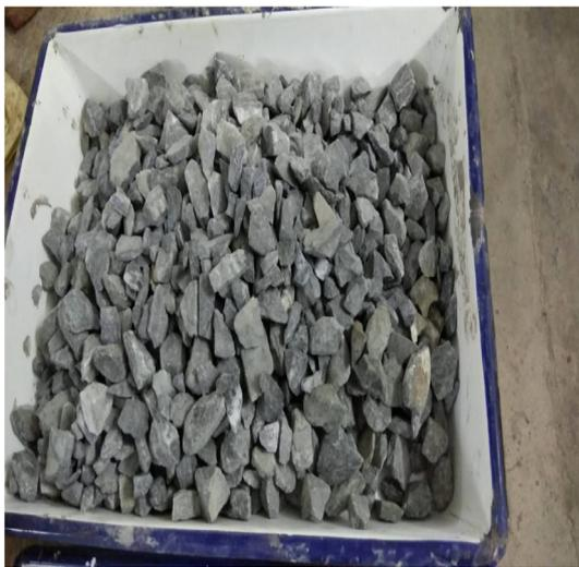
Fig. 3. Image of natural coarse aggregate.
