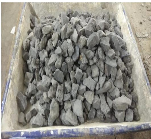
Fig. 4. Image of Ferrochrome slag aggregate.
