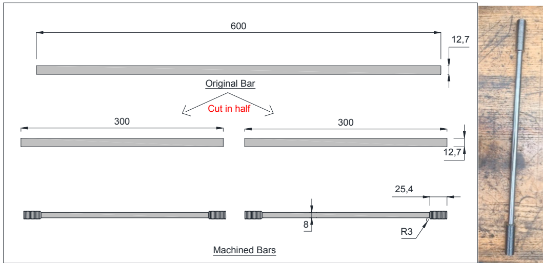
Fig. 3. SMA bar machining process.
