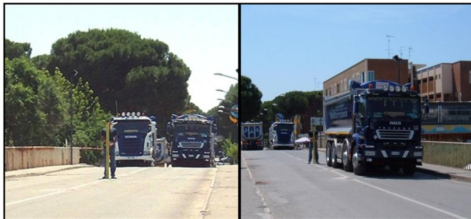
Fig. 4. Trucks in operation during the static load test.
