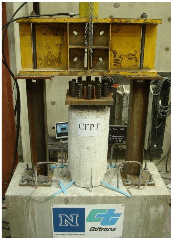
Fig. 5. Direct pull test setup for CFPT (image by Ali Mehrsoroush).
