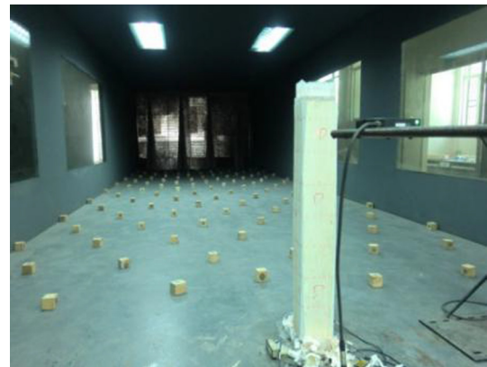
Fig. 7. Force vibration wind tunnel test photo.
