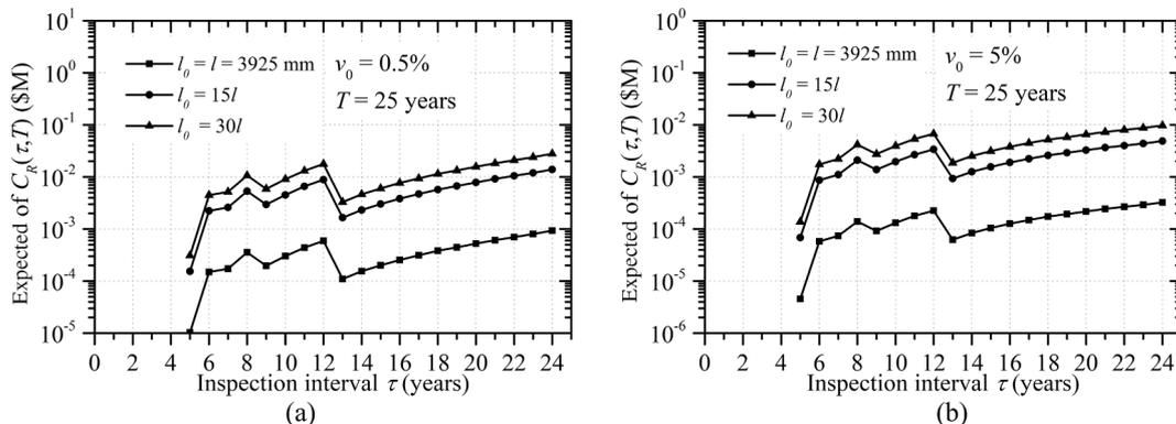
Fig. 5. Expected cost of structural renewal versus the inspection interval of dry-docking for  $T = 25$  years.  $l_0 = l = 3925$  mm,  $15l$ , and  $30l$  are considered for each case: (a)  $\nu_0 = 0.5\%$ ; (b)  $\nu_0 = 5\%$ .
