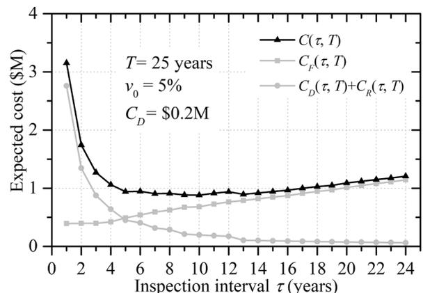
**Fig. 3.** Expected cost versus the inspection interval of dry-docking for the baseline example.
