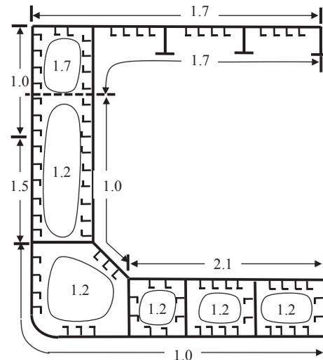
**Fig. 2.** Wastage allowance,  $t_{was}$ , at different ship locations (mm) (adapted from IACS [5]).
