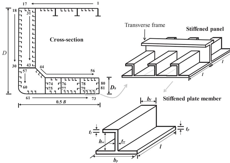
Fig. 1. Mid-ship cross-section of the tanker (adapted from [26]).
