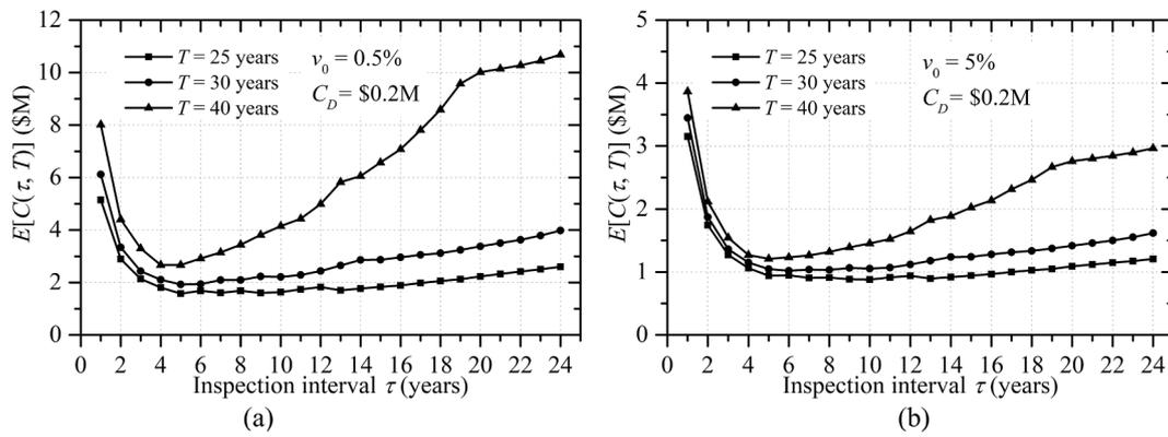
Fig. 4. Expected life-cycle cost versus the inspection interval of dry-docking for  $T = 25, 30,$  and  $40$  years: (a)  $\nu_0 = 0.5\%$ ; (b)  $\nu_0 = 5\%$ .
