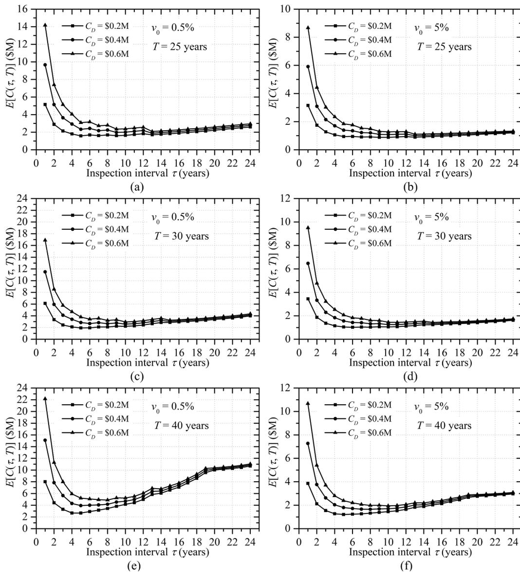
Fig. 6. Expected life-cycle cost versus the inspection interval of dry-docking for  $T = 25, 30,$  and  $40$  years, for different values of the life-cycle dry-docking cost  $C_D = \$0.2M, \$0.4M,$  and  $\$0.6M$ : (a), (c), (e)  $v_0 = 0.5\%$ ; (b), (d), (f)  $v_0 = 5\%$ .
