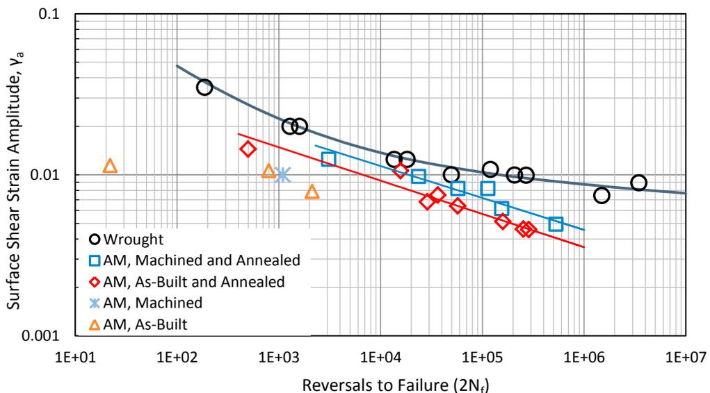
Fig. 7. Total shear strain amplitude vs. reversals to failure for fully-reversed torsional fatigue tests of wrought and AM Ti-6Al-4V with different heat treatment and surface finish conditions [26].
