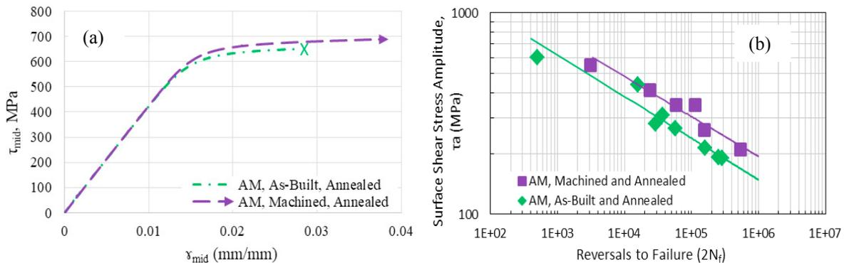
Fig. 5. Monotonic shear stress-strain curves (a) and shear stress amplitude vs. reversals to failure for fully-reversed torsional fatigue tests (b) of AM Ti-6Al-4V with machined and as-built surface finish conditions [26].
