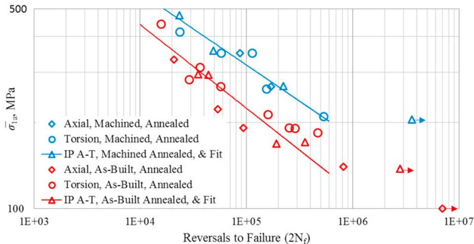
Fig. 8. Correlation of fatigue test results of PBF Ti-6Al-4V with different surface conditions based on maximum principal stress amplitude [4].
