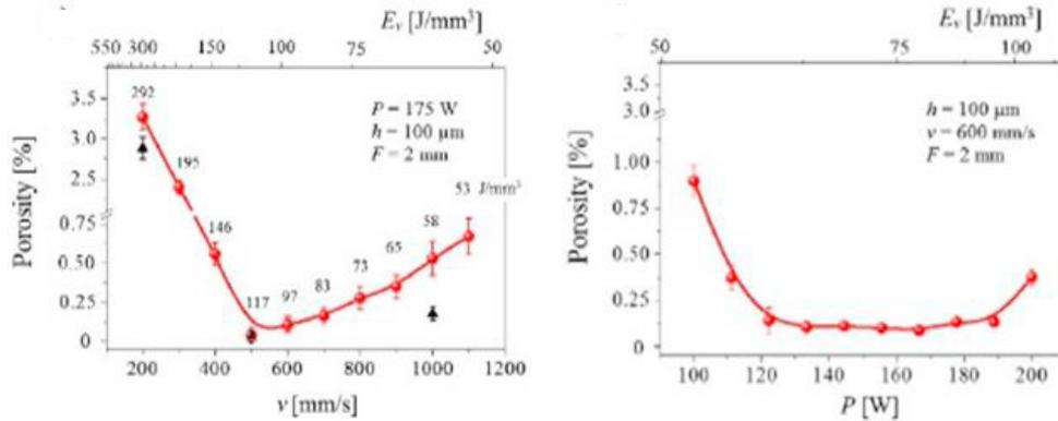
Fig. 2. Influence of the PBF process parameters on the amount of porosity for different parameter variations on Ti-6Al-4V samples. (a) Scanning velocity, and (b) laser power [9].
