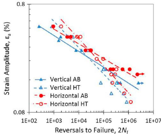
Fig. 4. Strain-life fatigue data for AM PBF 17-4 stainless steel in different build directions and with or without heat treatment [13].
