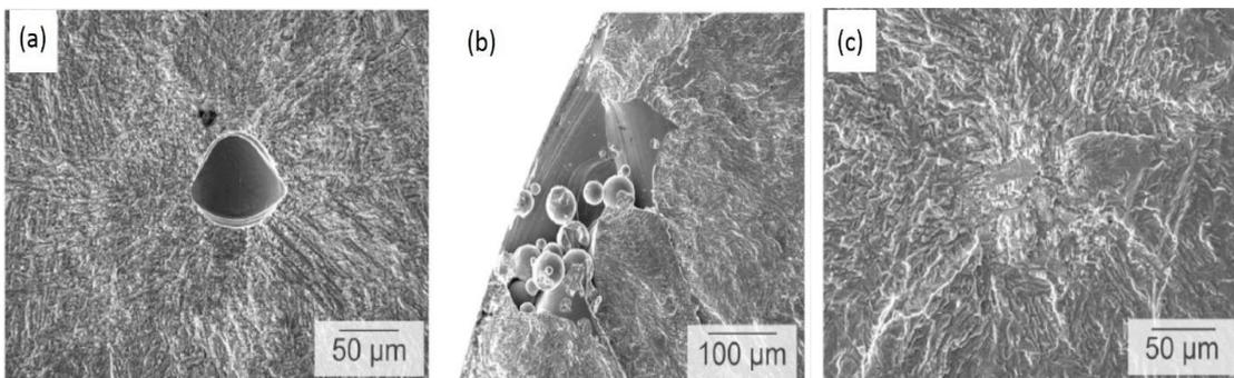
Fig. 1. Different representative defect types in AM Ti-6Al-4V: (a) Nearly spherical pore due to entrapped gas, (b) void due to un-melted particles, and (c)  $\alpha$ -phase grains defect [7].
