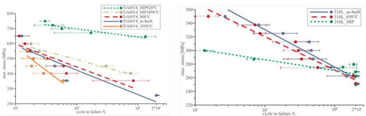
Fig. 6. S-N curves for PBF processed (a) Ti-6Al-4V, and (b) 316L under different heat treatment conditions [31].
