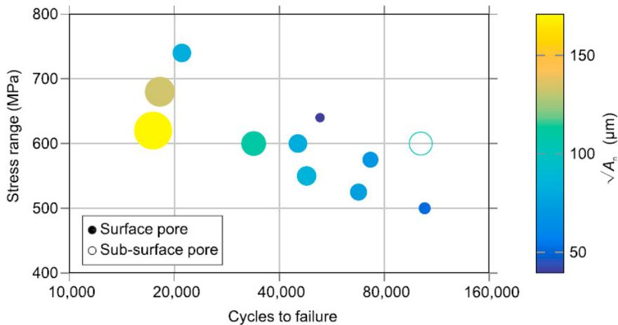
Fig. 3. Effect of pore size on fatigue life. The size and color of the markers indicate the size of the pore ( $A_n$ ) measured from SEM images of the fracture surface of EBM Ti-6Al-4V samples [12].
