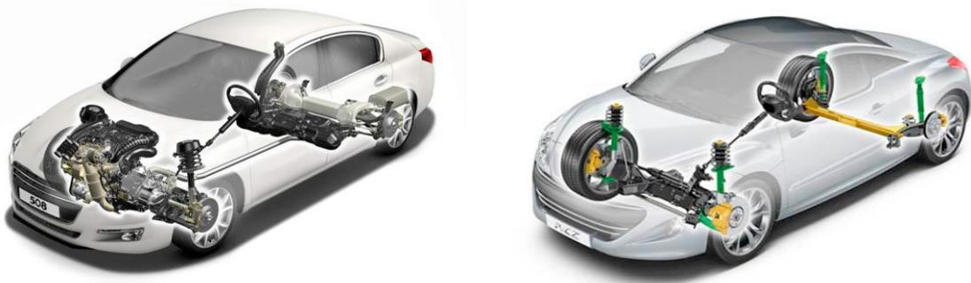
Fig. 1. Automotive chassis system: front and rear axles of a passenger car, Peugeot 508 (left) and Peugeot RCZ (right).
