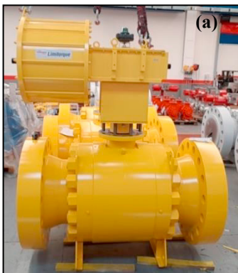
Figure 1: (a) LPS-30 actuator mounted on TMBCV Valbart valve, (b) Single acting fail close heavy-duty pneumatic actuator
