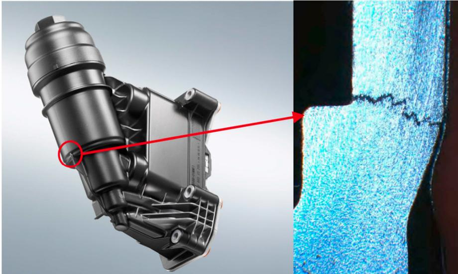
Figure 6: Application example: Oil-filter system at 150°C under pulsating pressure load, damage in test
