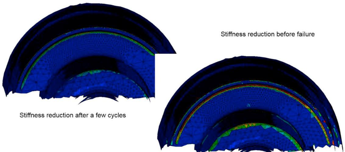
Figure 9: High stiffness reduction in the notch, leading to stress redistribution
