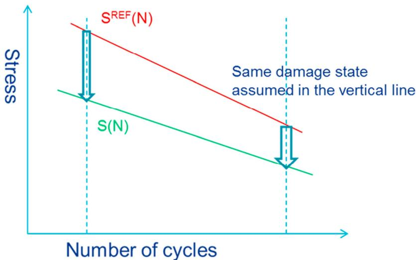
Figure 4: Idea of SN curve shift
