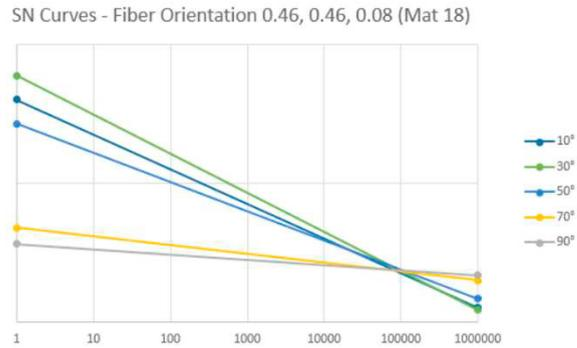
Figure 8: Orientation dependency of local SN curves
