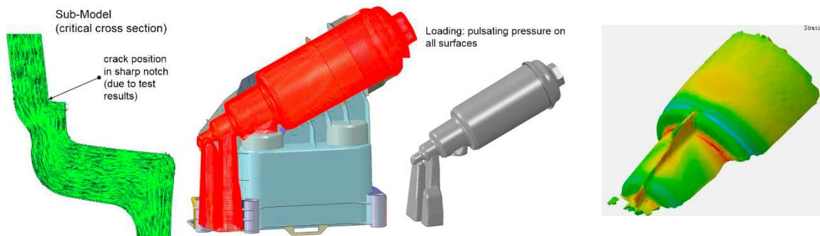
Figure 7: (a) Fiber distribution in the critical area, (b) Finite element model, (c) Stress results in LMS SAMCEF
