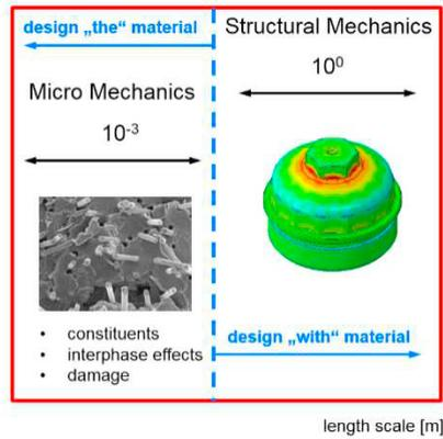
Figure 2: Micromechanics determines the behavior on the component level
