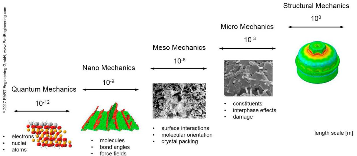
Figure 1: Different length scale domains of a material
