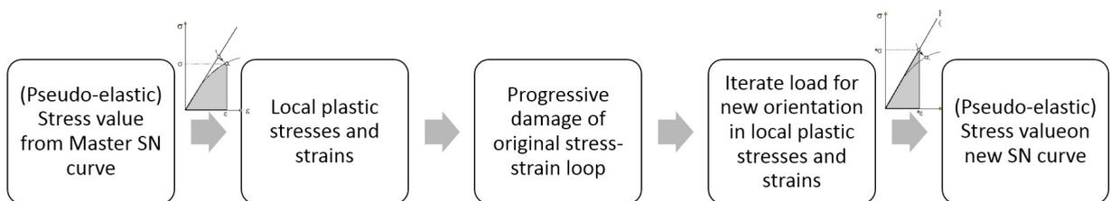
Figure 5: Process of the SN curve estimation using Neuber correction
