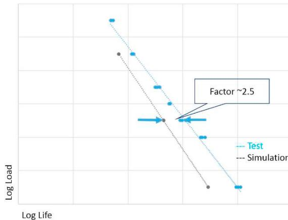
Figure 10: Comparison between simulated and tested life time.
