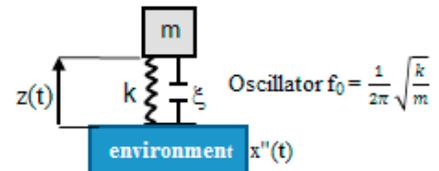
Assuming that the signal of environment is stationary and Gaussian, the displacement can be estimated in frequency domain with analytics calculus [8]
