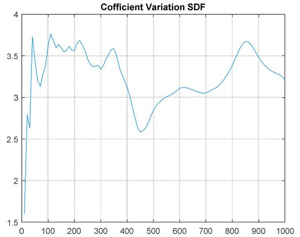
Fig 7: coefficient of variation of damages of the measured blocks – Tb = 5 s
