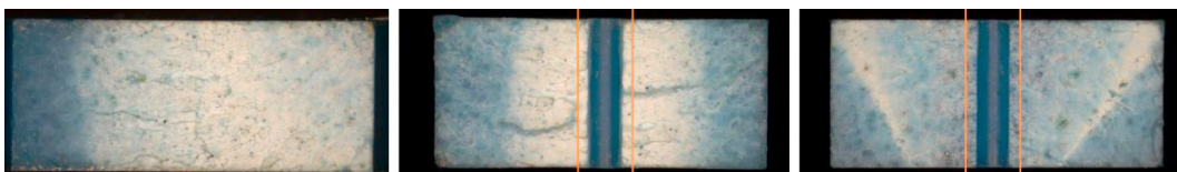
Fig. 12. Representative fracture surfaces of A3 adhesive: un-notched (left), notched-LCF (center) and notched-HCF (right)
