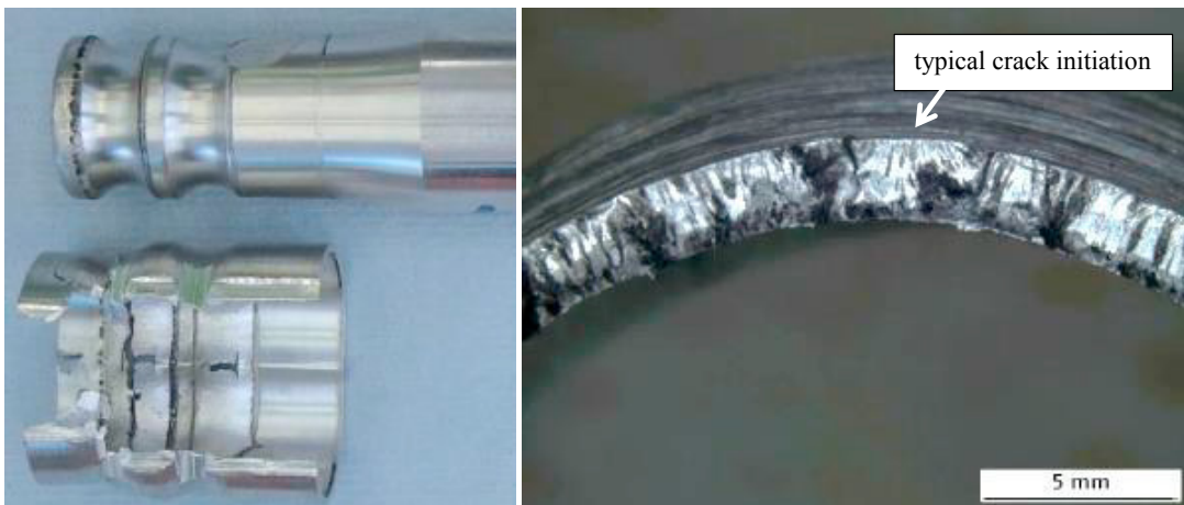
Fig. 12: Typical rupture (left) and fracture surface analysis (right)
