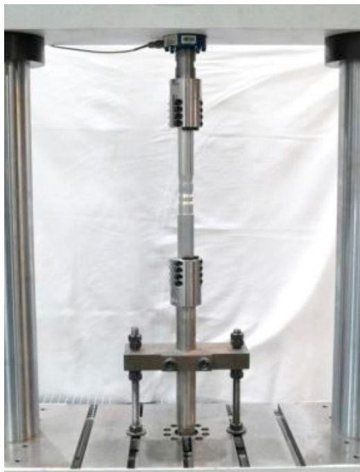
Fig. 6. Set-up for axial testing.
