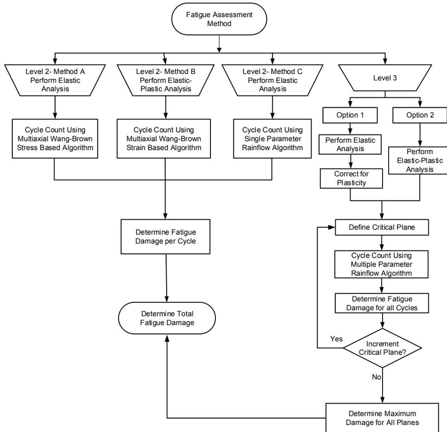
Figure 1. Fatigue analysis methods in API 579-1/ASME FFS-1
