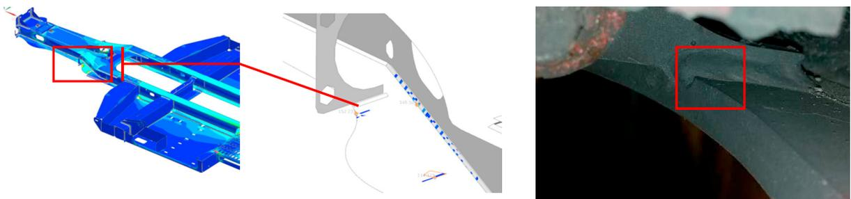
Fig.9. Drawbar support plate weld toe
