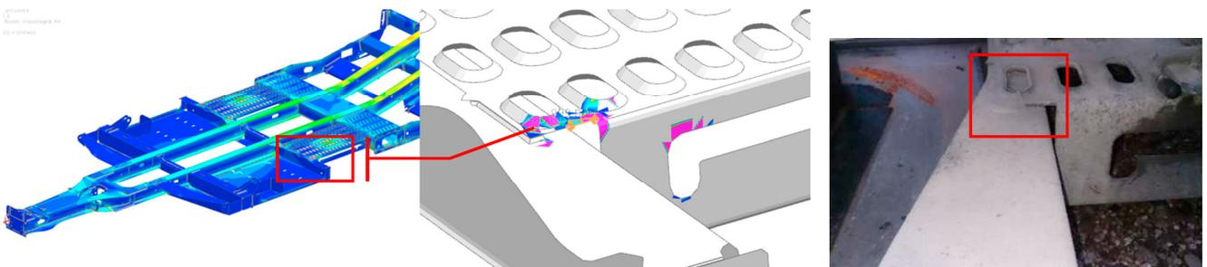
Fig.12. Chassis front platform
