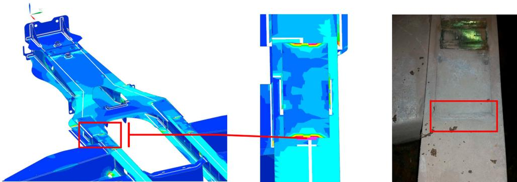
Fig.11. Chassis front cover plate
