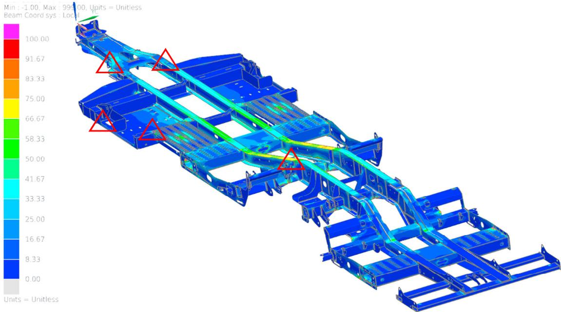
Fig.8. Trailer chassis fatigue results (%/fatigue limit)
