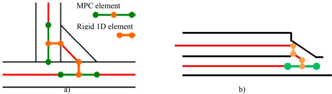
Fig. 5. Weld connectors a) T-joint b) overlap joint
