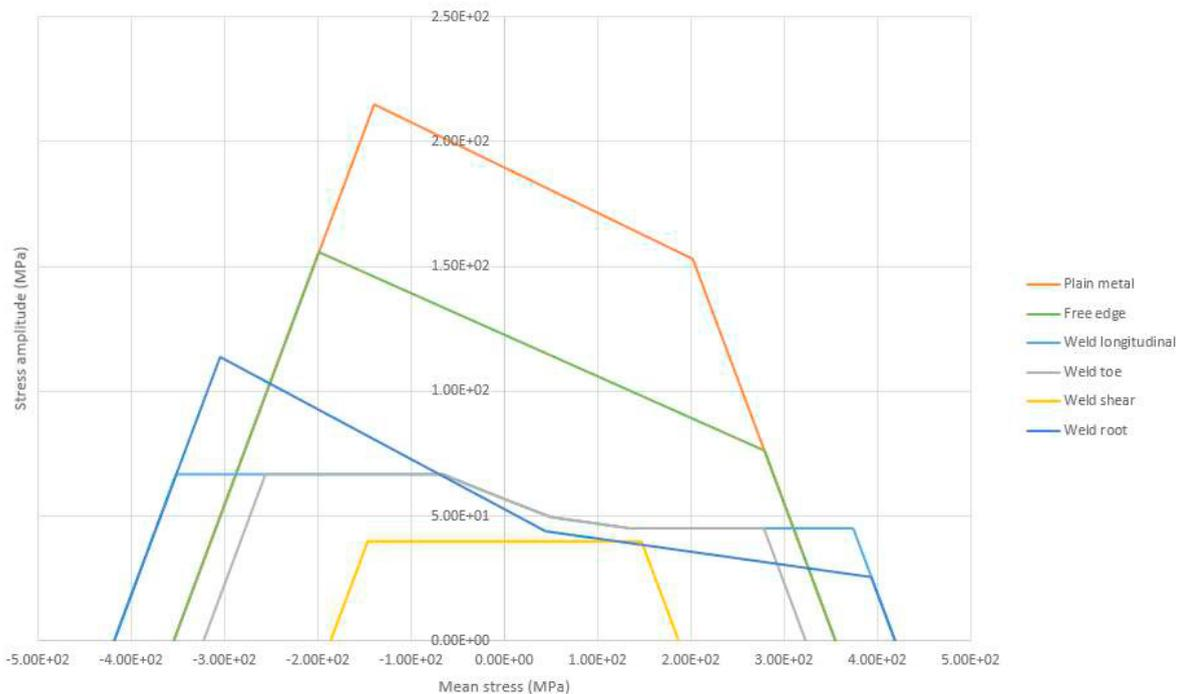
Fig. 7. Haigh diagrams according to the different zones of the model.
