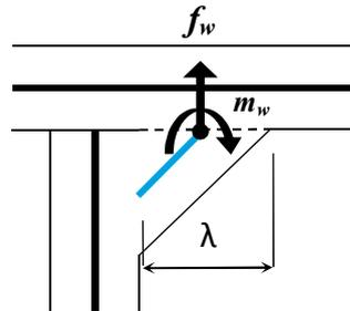
For weld toe, the structural fatigue stress limit is based on FAT 90 for load carrying fillet welds and FAT 100 for non-load carrying fillet welds and butt welds: S/N curves are given in [5]. FAT values correspond to admissible stress ranges for 2 million cycles with a survival probability of 97.5%. For weld root, the FAT curve for stress range is FAT 80 [4, 6, 7].
