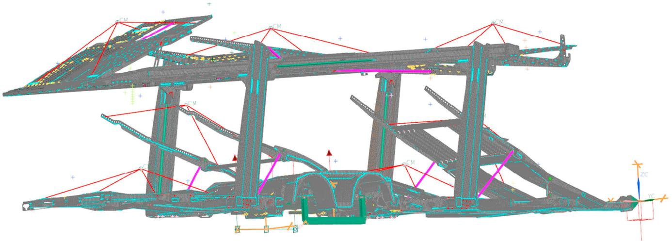
Fig. 6. Eurolohr 100 trailer structure FEA model
