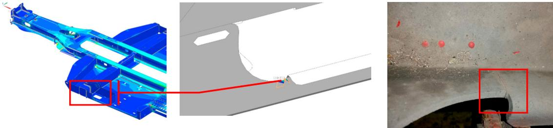
Fig.10. Front side fold
